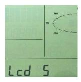
The LCD contrast can be set within 8 levels; from "Lcd 1" to "Lcd 8" (default setting is "Lcd 5"):
